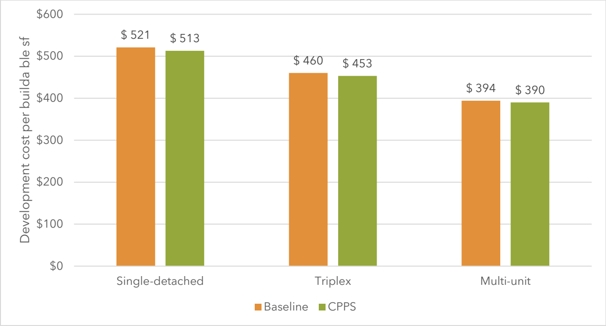
Figure 8: Development cost per buildable square foot for each scenario by housing type
